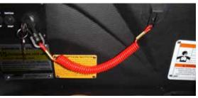
clip will pull free, pulling the switch to the OFF position. If the engine needs to be shut down very quickly, it can be done so by pulling on the lanyard to release it from the switch.
