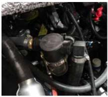
Raw water from the lake/river/sea is drawn into the boat to cool the engine and drive train. Even in closed cooling systems, it is necessary to circulate water in part of the system. To protect the system, an optional sea strainer may be installed near the raw water intake and serves the purpose of keeping debris from entering the cooling system and causing eventual engine failure. As with any kind of strainer, it is necessary to regularly clean it so that water can flow unimpeded.
