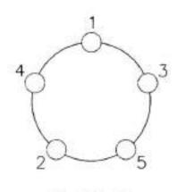
Follow these instructions for ensuring proper installation and torque for the lug nuts:
