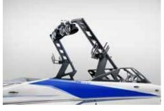
The tower on all Axis models is the Grey Skull. The Grey Skull can be raised to its full height for extraordinary boating enjoyment, or lowered for towing and storage, or for bridge clearance while on the water.
