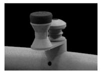
The optional tower lights are forward-facing. These lights can get hot with use. All tower lights are controlled through a toggle.
