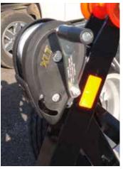
The trailer winch is a manually operated device to assist loading the boat onto the trailer and maintaining it in position for proper towing. The following information is important in assuring control and protection for you and the boat:
