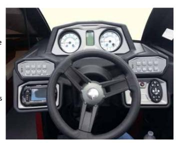
The Axis instrument panel features two (2) five-inch (5") gauges, which provide real-time information about important drive train functions.
