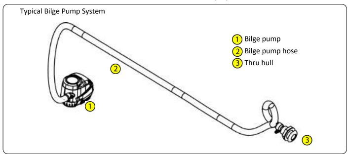
If water ever enters the forward part of the bilge, it can still be evacuated by the bilge pump. Located in the forward berth, there is an inspection plate, when removed, allows access to a drain plug. Simply remove the drain plug in the PVC pipe to allow the water to drain aft. Once all of the water has drained, re-install the drain plug.
