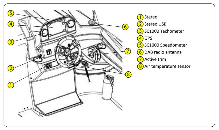
Please note that operator vision from the helm may be obstructed by high trim angles of the craft, along with other factors such as outboard engine trim angles, hull trim plane angles, loading and load distribution, speed & acceleration, transition from displacement to planing mode, sea conditions, rain and spray, darkness and fog, interior lights, position of tops and curtains, and persons or movable gear in the operator's field of vision.
