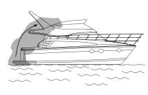
The station wagon effect or back drafting can cause CO gas to accumulate inside the cabin, cockpit or bridge areas when the boat is underway using protective weather coverings. PRECAUTION: Provide adequate ventilation when the canvas top, side or back curtains are in their closed, protective positions. Open forward hatch or window.
