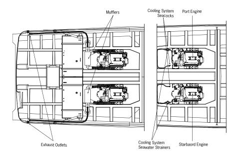
can flood the non-running engine with seawater, damaging it. Before you restart the non-running engine, open its seacock again.
