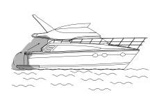
CO gas can accumulate in the cabin, cockpit and bridge areas when operating your boat at slow speeds or when the boat is stopped in the water. A tail wind can also increase accumulation (force of wind entering from aft section of yacht).
