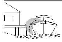
Blockage of exhaust outlets can cause carbon monoxide to accumulate in the cabin and cockpit area - even when the hatches, windows, portholes and doors are closed.
