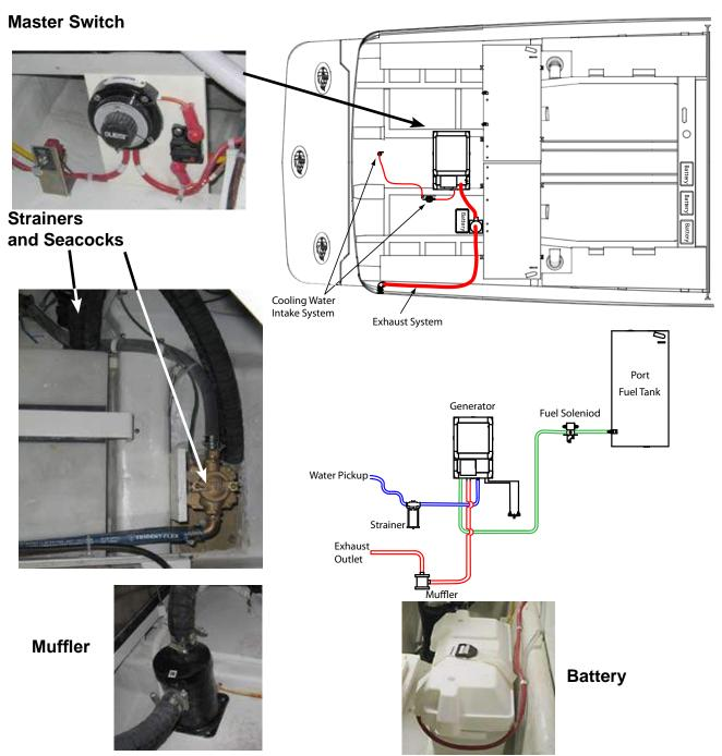
2. The generator starter is powered by its own 12-volt battery. Turn the generator battery master disconnect switch to the ON position.
