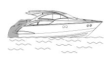
CO gas can accumulate in the cabin, cockpit and bridge areas when operating your boat at slow speeds or when the boat is stopped in the water. A tail wind can also increase accumulation (force of wind entering from aft section of yacht).
