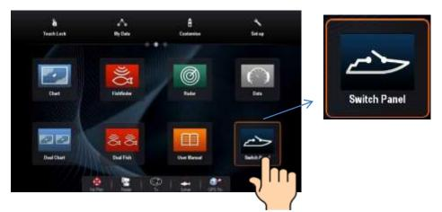
The Switch Panel for the 24 Resorter provides control of most of the vessel's electrical systems via touchscreen interface.
