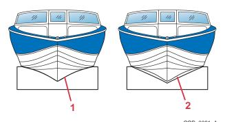
1 - Hull completely on cradle - right
