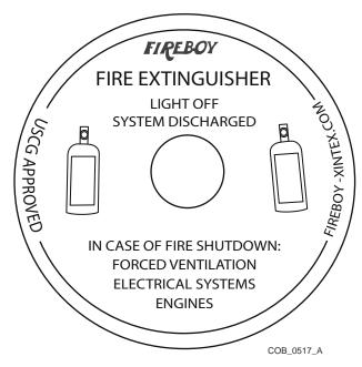
Inspect fire extinguishers for proper charge before operating the boat.
