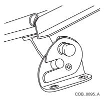
To close the windshield, release the locking mechanism by pulling the forward-facing button. Swing the windshield into place.
