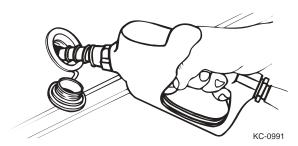
When your boat is equipped with the pop-up fuel filler cap, open by pressing the cap and turning the cap counterclockwise (approximately 10°); remove cap.
