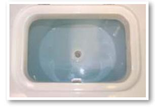
through the grate on the top of the standpipe, which, when unobstructed, will limit the water level to the standpipe's highest point. A shorter standpipe can be used to keep less water in the well. This constant drainage keeps up water flow and allows for the removal of ammonia from the livewell, therefore extending the life of your baitfish. To drain the livewell, switch off the pump, close pump ball valve, and remove standpipe.
