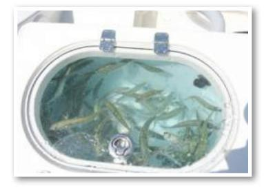
standpipe's highest point. A shorter standpipe can be used to keep less water in the well. This constant drainage keeps up water flow and allows for the removal of ammonia from the livewell, therefore extending the life of your baitfish. To drain the livewell, switch off the pump, close pump ball valve, and remove standpipe.
