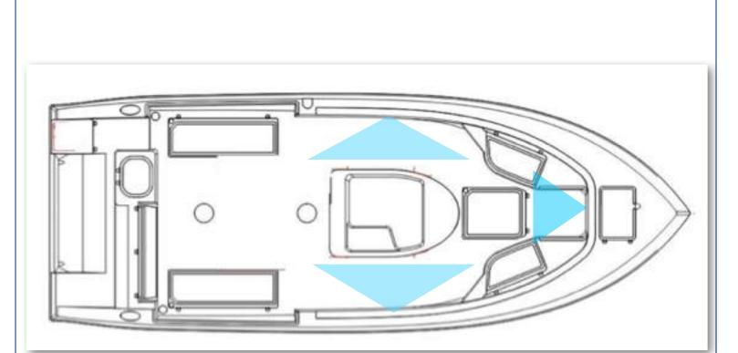
Diagram of the LED Cockpit Courtesy Lights
