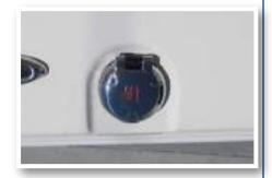
The fuel sending unit and fuel pick up on the tank can be accessed at the pie hole on the cockpit floor behind the leaning post. The fuel vent and the fuel fill at the tank can be accessed at the pie hole forward of the leaning post.
