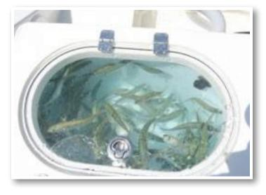
water in the well. This constant drainage keeps up water flow and allows for the removal of ammonia from the livewell, therefore extending the life of your baitfish. To drain the livewell, switch off the pump, close pump ball valve, and remove standpipe.
