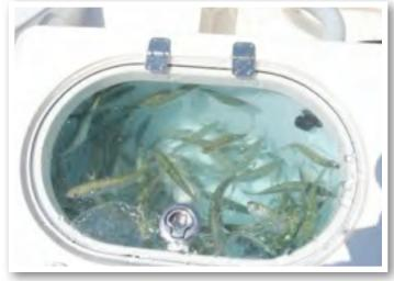
keep less water in the well. This constant drainage keeps up water flow and allows for the removal of ammonia from the livewell, therefore extending the life of your baitfish. To drain the livewell, switch off the pump, close pump ball valve, and remove standpipe.
