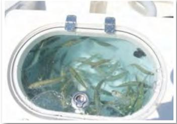
achieved through the grate on the top of the standpipe. This constant drainage keeps up water flow and allows for the removal of ammonia from the livewell, therefore extending the life of your baitfish even further. To drain the livewell, switch off the pump, close pump ball valve, and remove standpipe.
