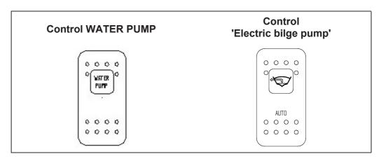
On the electrical panel - three possible positions : OFF / Automatic / Mechanically operated. In the automatic position each pump is set off automatically by a trip switch located in the sump area or in the bottom of the hull.
