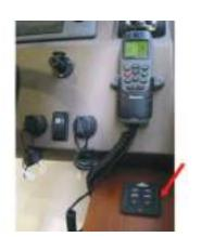
Location Control box: Engine compartment
