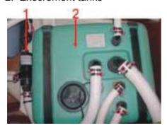
Gauge + Tank discharge switch to sea
