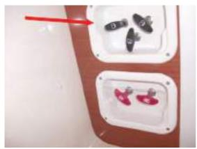
Remote pull switches - Supply tanks + generator
