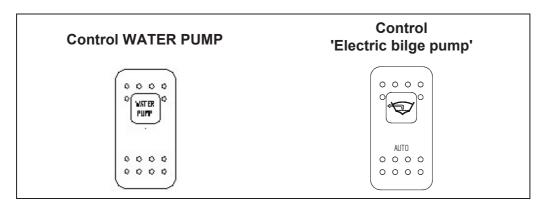
On the electrical panel - three possible positions : OFF / Automatic / Mechanically operated.
