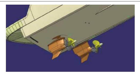
Steering is obtained through rotation of the IPS housings.
