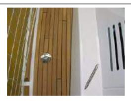
Drainage Tank - Filler cap (Port catwalk)
