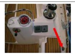
Filler cap - Starboard catwalk
