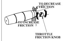
Use the throttle friction knob to help hold a constant throttle setting while cruising.
