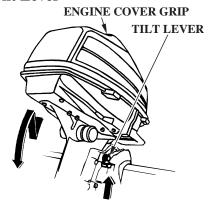
The tilt lever enables the outboard motor to be raised for shallow water operation, beaching, launching, or mooring.
