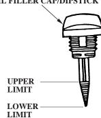
4. If the oil level is low, add oil to reach the upper limit mark shown on the dipstick. Use the oil recommended on p. 45.
