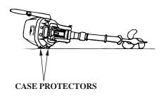
If storing horizontally, be sure to fold the tiller handle, and rest the outboard motor on its case protectors. Be sure all water has drained from the outboard motor before placing it on its side, so no residual water can enter the engine exhaust port.
