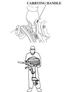
To carry, hold the outboard motor by the carrying handle, or hold by the carrying handle and the lug beneath the engine cover lock latch, as shown.
