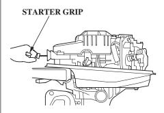
4. Remove the spark plug (p. 49), and remove the emergency stop switch clip from the emergency stop switch. Pull the starter grip, rotate the flywheel a few revolutions to completely expel any water from the cylinder.
