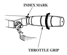
The throttle grip controls engine speed.
