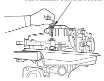
3. Insert the dipstick without screwing it in, then remove it and check the oil level shown on the dipstick.
