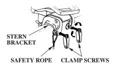
Attach the stern bracket to the boat transom by tightening the clamp screws.
