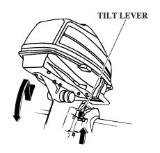
To return the outboard motor to the normal operating position, raise the outboard slightly by pulling on the engine cover grip, then pull the tilt lever to release the outboard, and then slowly lower the outboard motor.
