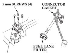
FUEL TANK FILTER JOINT (Fuel Hose Connector)
