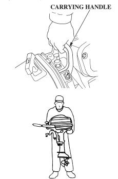
To carry the outboard motor, hold it by the carrying handle, or hold by the carrying handle and the lug beneath the engine cover lock lever, as shown.
