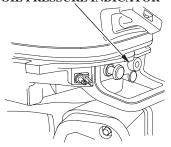
When the oil pressure indicator is lit, oil pressure is OK.
