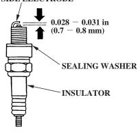
5. Measure the spark plug electrode gap with a wire-type feeler gauge. Correct the gap, if necessary, by carefully bending the side electrode.
