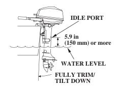
Adverse effect to the engine can occur if the installation position of the outboard motor is too low. Trim/tilt down the outboard motor with the boat fully loaded and stop the engine. Check that the idle port is 5.9 in (150 mm) or more above the water level.
