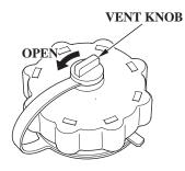
2. Turn the fuel filler cap counterclockwise so that it touches the pressure relief tab.
