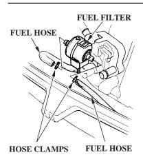
4. Remove the fuel hoses from the used filter, and discard the filter.
