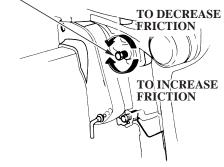
Use the steering friction bolt to help hold a steady course while cruising.
