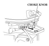
3. To start a cold engine, pull the choke knob to the ON position. To restart a warm engine, leave the choke knob in the OFF position.
