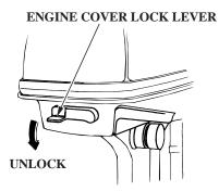
The engine cover lock lever fastens the engine cover to the outboard motor.
