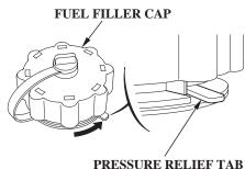
3. Press down the pressure relief tab, and then turn the fuel filler cap 1/4 counterclockwise. Release the pressure relief tab. Wait to relieve pressure.
