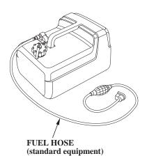
The portable fuel tank has a capacity of 3.2 US gal (12L) and has a fuel gauge built into the fuel tank connector.
