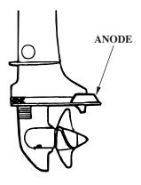
The anode is made of a sacrificial material that helps to protect the outboard motor from corrosion.
