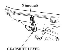
2. Check the position of the gearshift lever. It must be in the N (neutral) position for starting.
