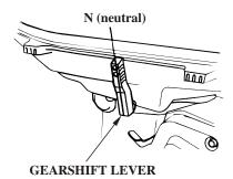
1. Move the throttle grip to the slowest speed and gearshift lever to the N (neutral) position.
