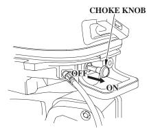
The choke knob opens and closes the choke valve in the carburetor.
