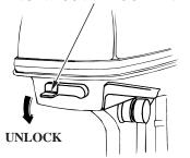
1. Unlock and remove the engine cover.
