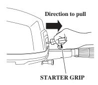
Pulling the starter grip operates the recoil starter to crank the engine for starting.
