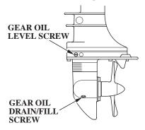
Remove the oil level screw and see whether oil flows from the oil level hole.
