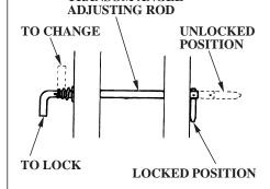
The transom angle adjusting rod is used to adjust the angle of the outboard motor in the normal operating position (p. 35).
