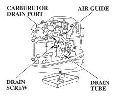
3. With the outboard motor in a vertical position, place an approved gasoline container below the fuel drain outlet, and use a funnel to avoid spilling fuel.
