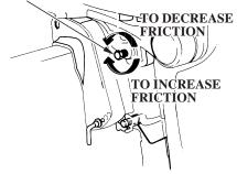
The steering friction bolt adjusts steering resistance.
