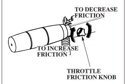
The throttle friction knob adjusts resistance to throttle grip rotation.
