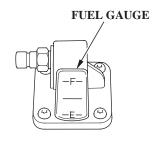
A fuel gauge is built into the fuel tank connector of the portable fuel tank.
