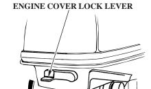
1. Unlock and remove the engine cover for access to the fuel pump filter.
