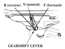
To shift gears, turn the throttle grip to the SLOW position; then move the gearshift lever to select the F (forward), N (neutral), or R (reverse) gears.
