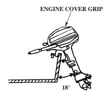
To tilt the outboard motor, raise the outboard motor to the 30° position by pulling on the engine cover grip.
