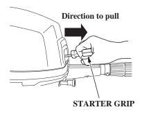
5. Pull the starter grip lightly until you feel resistance, then pull briskly in the direction of the arrow as shown above.
