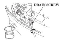
2. With the outboard motor in a vertical position, place an approved gasoline container below the fuel drain outlet, and use a funnel to avoid spilling fuel.
