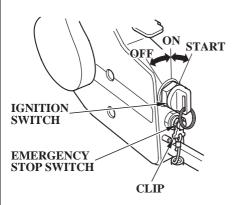
The ignition switch controls the ignition system and starter motor.
