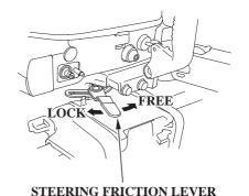
The steering friction lever adjusts steering resistance.
