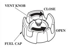
To refuel, turn the vent knob counterclockwise to the OPEN position, and unscrew the fuel tank cap.
