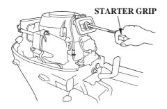
4. Remove the spark plugs (p. 61), and remove the clip from the emergency stop or engine switch. Pull the recoil starter grip, rotate the flywheel a few revolutions to completely expel any water from the cylinders.
