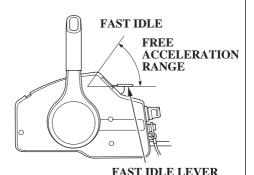
3. To start a cold engine, leave the fast idle lever in the OFF (fully lowered) position.
