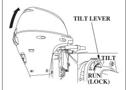
The tilt lever enables the outboard motor to be raised for shallow water operation, beaching, launching, or mooring.
