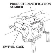
The product identification number is stamped on a plate attached on top of the stern bracket.
