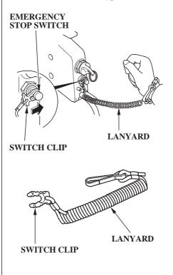
The switch clip must be inserted in the emergency stop switch in order for the engine to start and run. The lanyard must be attached to the operator's PFD (Personal Flotation Device) or worn around the wrist as shown.
