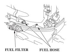
4. Remove the fuel tubes from the used filter, and discard the filter.
