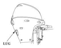
To carry, hold the outboard motor by the carrying handle, or hold by the carrying handle and the lug beneath engine cover lock lever, as shown.
