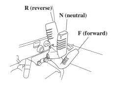
The gearshift lever is used to select F (forward), N (neutral), or R (reverse) gears.
