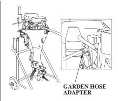
After flushing, remove the garden hose adapter, reinstall the engine cover.
