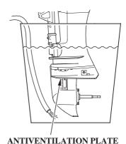
1. Place a container under the outboard motor, and fill it with clean, fresh water. The water level must be at least 2 inches above the antiventilation plate.
