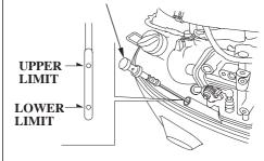
3. Insert the dipstick all the way in, then remove it and check the oil level shown on the dipstick.
