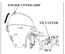
To return the outboard motor to the normal operating position, move the tilt lever to the RUN position, raise the outboard motor slightly to disengage the tilt mechanism, then slowly lower the outboard motor.
