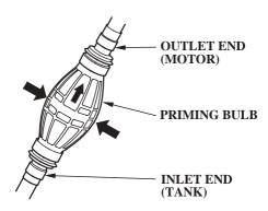
Hold the priming bulb with the outlet end higher than the inlet end. Squeeze the priming bulb several times, until it feels firm, indicating that fuel has reached the carburetor.
