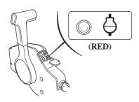
If the engine overheats, the red light will come on, and the engine protection system will limit engine speed.
