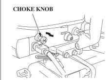
The choke knob opens and closes the choke valves in the carburetors.
