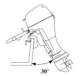
To tilt the outboard motor, move the tilt lever to the TILT position, then raise the outboard motor to the 30° or 45° position by pulling on the engine cover grip.
