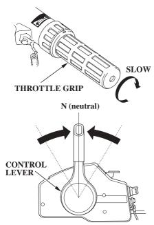
1. Move the throttle grip to the slowest speed and control gears to N (neutral) position.
