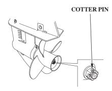
Remove the cotter pin, unscrew the castle nut, remove the washer, then remove the propeller and thrust washer.
