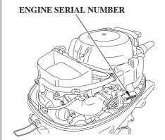
The engine serial number is stamped on the right front of the engine.
