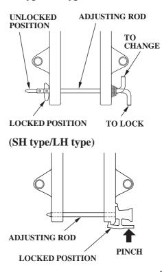
The transom angle adjusting rod limits the tilt angle of the outboard motor when fully lowered.
