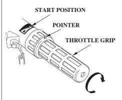
4. Do not turn the throttle grip before starting and align the START position with the pointer for starting the engine.
