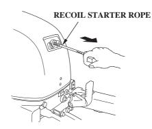
Inspect the recoil starter rope, and replace it if it becomes frayed.
