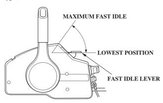
The fast idle lever is provided with the engine idle speed adjusting function.
