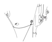
ENGINE OIL DRAIN SCREW
