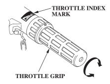
The throttle grip controls engine speed.
