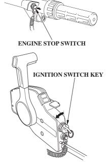
2. Turn the ignition switch key to the OFF position or press the engine stop switch until the engine stops.
