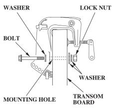
Attach the stern bracket to the boat transom by tightening the clamp screws.
