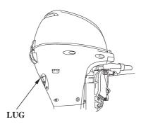
To carry the outboard motor, hold it by the carrying handle, or hold by the carrying handle and the lug beneath the engine cover latch, as shown.
