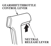
The control lever automatically locks itself in the N (neutral) position. To move the lever out of the N (neutral) position, you must squeeze the neutral release lever on the underside of the lever handle.
