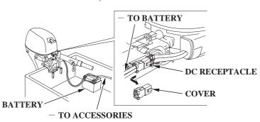
To prepare the outboard motor for connection to a battery, pull the cover out of the DC receptacle, connect your battery charging wires to the receptacle. Attach the connected DC receptacle on the holder on the tiller arm.
