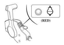
If the engine overheats, the red indicator light will come on, and the engine protection system will limit engine speed. If you are at cruising speed, engine speed will decrease gradually.
