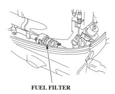
2. Inspect the filter for water and/or sediment accumulation.
