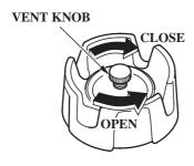
The cap is provided with a vent knob to seal the portable fuel tank for carrying it to and from the boat. Open the vent knob 2 or 3 turns before starting the engine (p. 34).
