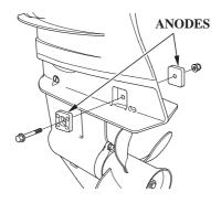
The anodes are located on each side of the gearcase. They are made of a sacrificial material that helps to protect the outboard motor from corrosion.
