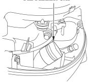
4. If the oil level is low, remove the oil filler cap, and add oil to reach the upper limit mark shown on the dipstick. Use the oil recommended on p. 59.
