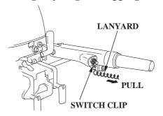
To stop the engine in an emergency, pull the clip out of the engine or emergency stop switch by pulling the lanyard.
