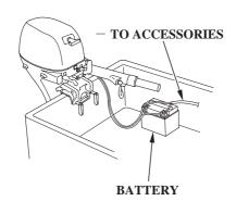
Honda BF8D/BFP8D/BF9.9D and BFP9.9D outboard motors produce a 12-volt, 12-ampere battery-charging current and are equipped for connection to a 12-volt battery. The battery-charging circuit is protected by a 20-ampere fuse located in the engine compartment.
