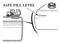
Refuel in a well-ventilated area. Fill the tank to the SAFE FILL LEVEL line.
