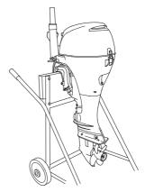
Store the outboard motor either vertically or horizontally with the tiller handle side up.
