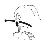
To shift gears, move the control lever to select F (forward), N (neutral) and R (reverse) gears.
