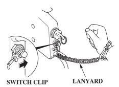
1. Put the emergency stop switch clip in the emergency stop switch, and attach the lanyard to your PFD (Personal Flotation Device) or to your wrist, as shown. The engine will not start or run, unless the clip is in the switch.
