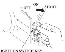
4. Turn the ignition switch key to the START position and hold it there until the engine starts.
