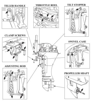
Apply Honda Marine Corrosion Inhibitor (or equivalent) to all areas under the engine cover except the belts.
