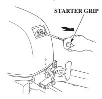
Pull the starter grip to operate the recoil starter for starting the engine manually.
