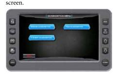
When choosing this selection, the display will query the engine(s) ECU, as illustrated below, and provide feedback.
