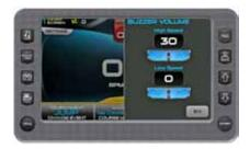
Touch [Settings]. Touch [Buzzer Vol**ume**]. On the Pop-up, touch the arrows to set a value at high speed and low speed.
