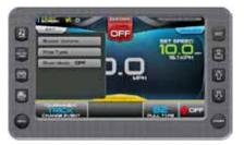
Touch [Settings]. Touch [River Mode] to select ON or OFF. With River Mode ON, touch to set the River Dir Offset UP and DOWN values using the arrows.
