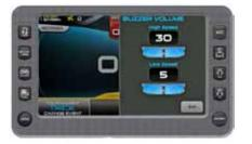
Touch [Settings]. Touch [Buzzer Volume]. On the Pop-up, touch the arrows to set a value at high speed and low speed.
