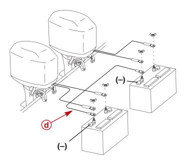
d - Ground Cable (Same Wire Size As Engine Battery Cable) – Connect Between Negative (–) Terminals
