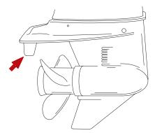
**NOTE:** Trim tab adjustment will have little effect reducing steering torque if the anti-ventilation plate is raised 2 inches (50mm) or more above the boat bottom.
