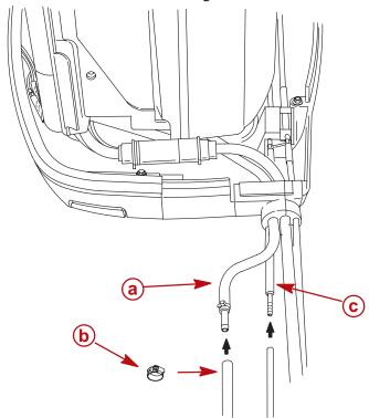
**NOTE:** If the speedometer water pick-up hose is not used, keep the hose routed out of the rubber grommet.
