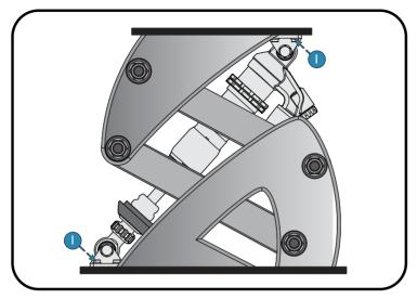
1. The seat height can be adjustable by moving these fasteners back or forward
