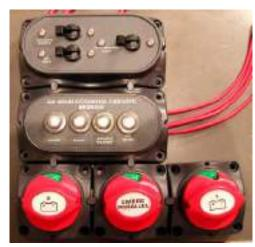
Battery Switches and Main Breakers
