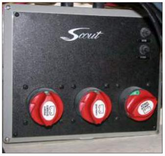
Twin Engine Battery Switch Panel
