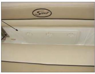
Aft Electrical Systems Compartment Hatch Behind Stern Bench Seat
