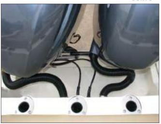
Typical Twin Engine Steering Cylinders & Tie Bar
