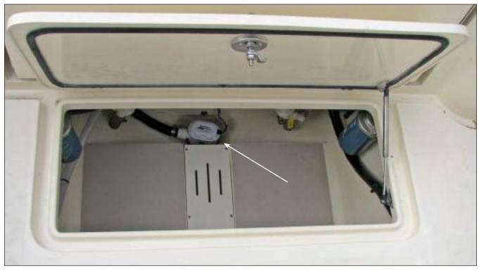
Aft systems compartment Showing Hatch Drain Rails & Bilge Pump
