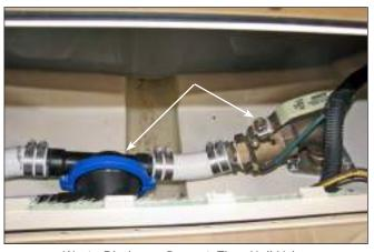
Waste Discharge Pump & Thru-Hull Valve
