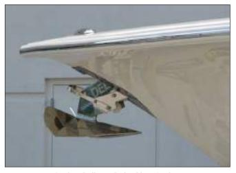
Anchor Roller & Delta Plow Anchor
