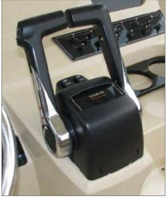
Typical Twin Engine Cable Controls
