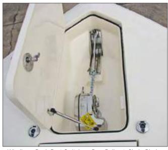
Windlass, Deck Foot Switches, Bow Roller & Chain Binder
