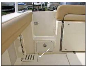
Starboard Cockpit Scupper Drain
