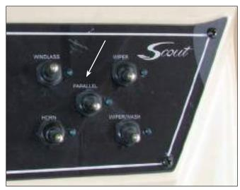
Parallel Switch In Helm Switch Panel
