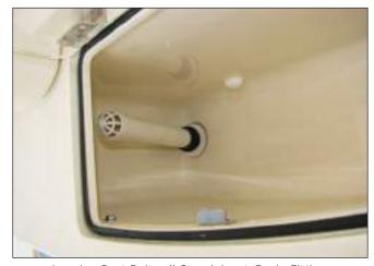
Leaning Post Baitwell Standpipe & Drain Fitting
