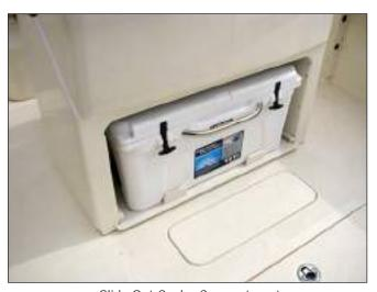
Slide Out Cooler Compartment & Fuel Sending Unit Access Hatch
