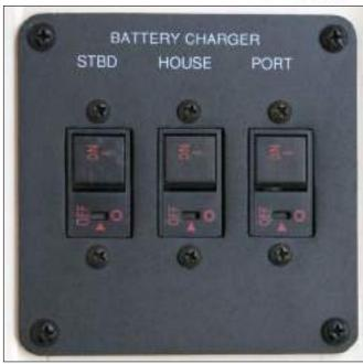
Twin Engine External Battery Charging Circuit Protection
