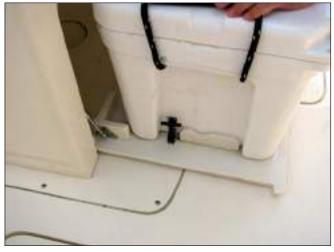
Cooler Slide Assembly & Draw Latch
