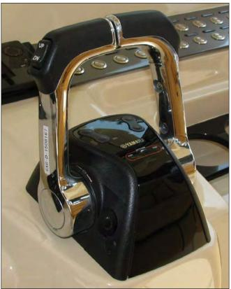
Typical Yamaha Twin Engine Electronic Controls
