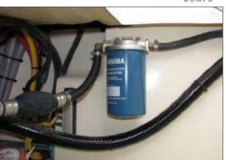
Engine Fuel Filter & Primer Bulb In Aft Systems Station
