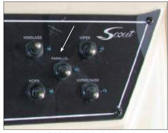
Parallel Switch In Helm Switch Panel
