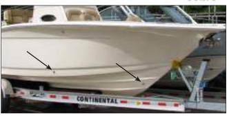
Forward Fishbox/Storage Compartment & Rope Locker Drains
