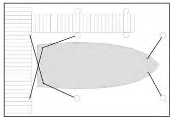
Securing Boat In A Slip (Typical)
