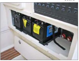
Typical Twin Engine Batteries
