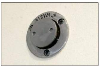
Waste Deck Fitting - Cap Released & Providing Handhold Note: Press down and turn cap 1/4 turn counter-clockwise to release and provide handhold.
