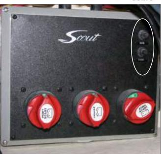
Twin Engine Battery Switch Circuit Breakers
