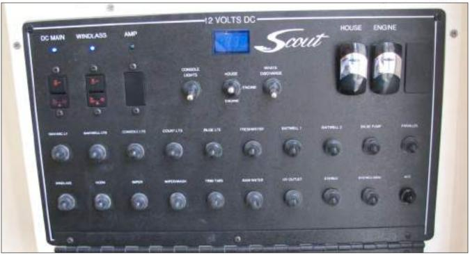
DC Breaker Panel & Remote Battery Switches
