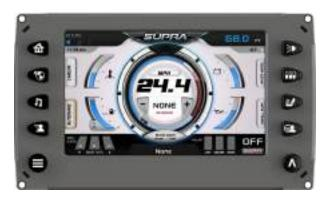
The cruise control can be turned ON or OFF from this screen by touching **[ZEROOFF]** located in the lower right of the screen.
