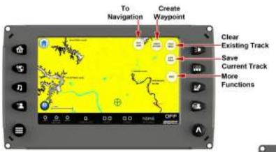
Touch [CREATE WAYPOINT] to add a waypoint to the map. A keypad is displayed to type the name (10 alpha character limit). When finished typing the name touch [DONE].
