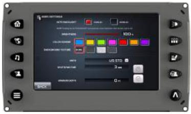
To edit the settings, touch the field to be changed. For Shutdown Time and Minimum Depth, touch the or arrows to adjust the settings. Touch [Back] to save the settings and return to the Main Menu screen.
