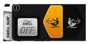
Swell Surf will cause the trim plates to deploy to create a surfing swell on the side the rider is surfing. Touch the Off button to turn the system on then touch the side on which the surfing will occur.
