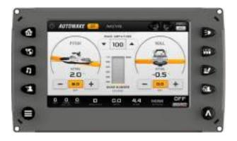
the home screen. Select either Save to Current Profile or Save to New Profile. Each rider can have differing set points for Surf Port and Surf Starboard. The Amplitude Potential bar is used to achieve the optimal surf number and wave size.
