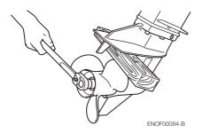
6. Install a new split pin into the nut hole and bend it.
