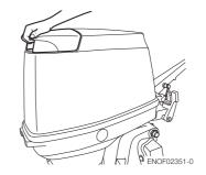
Push the reverse lock lever downward until it stops.(this is the tilt LOCK position.)
