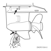
Install the upper oil plug, and then remove oil tube nozzle and install the lower oil plug.
