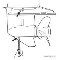
Insert the oil tube nozzle into the lower oil plug hole, and fill with gear oil by squeezing the oil tube until oil flows out of the upper plug hole and bubbles is disappeared to remove the air.
