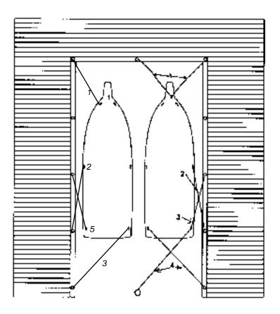
The two spring lines are crossed and running to separate deck cleats. If possible, the stern line should be run to the offshore quarter cleat. Spring lines are useful in preventing undesired movement ahead or astern in a berth; they also keep a moored vessel in position when there is a significant rise or fall in tide.
