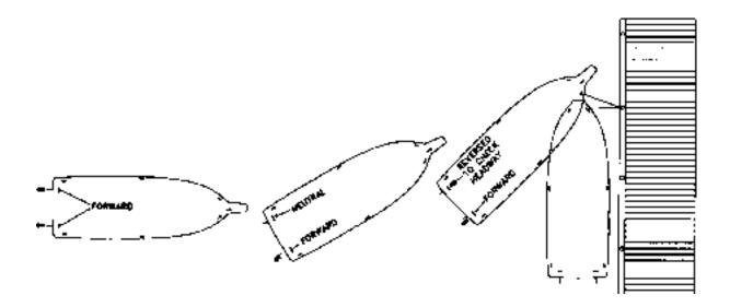
engine to check headway. Leave the starboard engine in forward gear to swing the boat parallel to the pier. For landings on the port side, turn the rudders to starboard and put the starboard engine into reverse as the boat comes in. You may have to shift into and out of gear to control the boat's speed.
