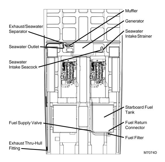
Operate the blowers for at least 4 minutes and until the engine room is free of any fuel vapor before starting the generator. Continue operating the blowers while the generator is running.
