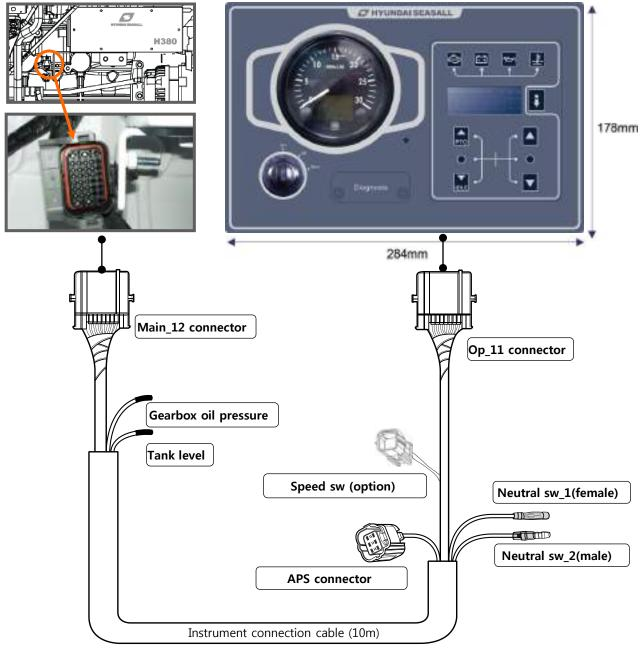
If there is no neutral switch, you must connect the neutral switch-1 and neutral switch-2 of the instrument connection cable.
